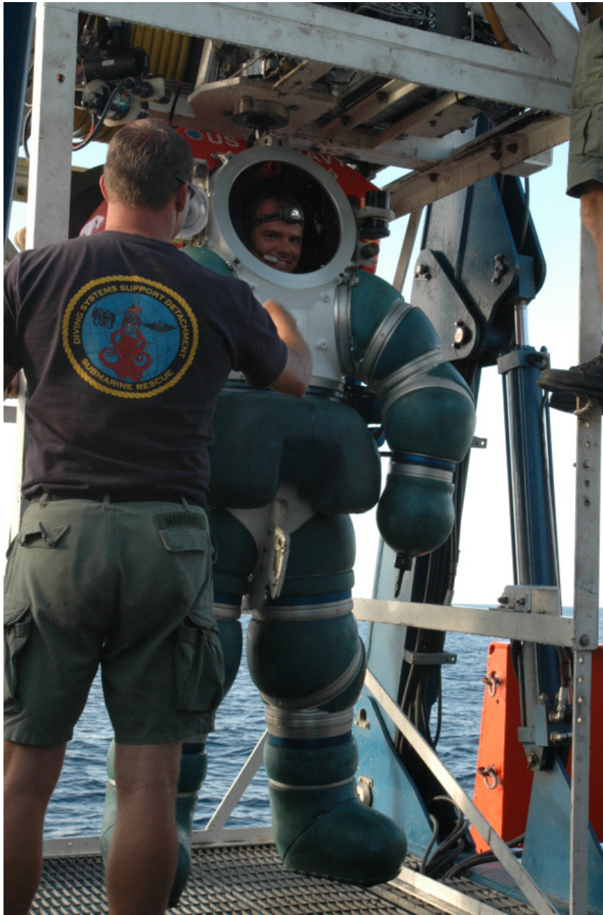
Chief Navy Diver Daniel Jackson completes a successful dive using a modern ADS. This system still uses the rudimentary pincers developed for the Navy over a century ago. (Photo by Mass Communication Specialist Seaman Chelsea Kennedy)
